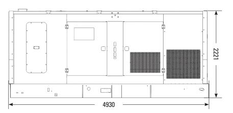
Approximate weight of enclosure package: 4667 kg (10289 lb), \*\*4770 kg (10516 lb) DE450E3. Exact weight is dependent on options. Enclosure weight includes: Sound attenuated enclosure, exhaust system, base and generator set.
