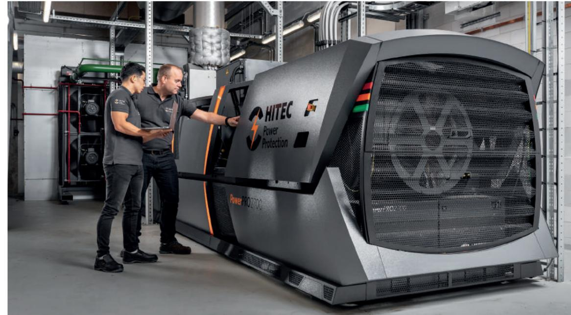
The unique line-interactive concept of a HITEC UPS offers significant benefits. The UPS does not perform the double energy conversion that a battery UPS must execute as soon as the utility power degrades or falls outside specified limits. No power electronics are utilized within the HITEC system; instead, the incorporated synchronous generator is used to supply the load.
