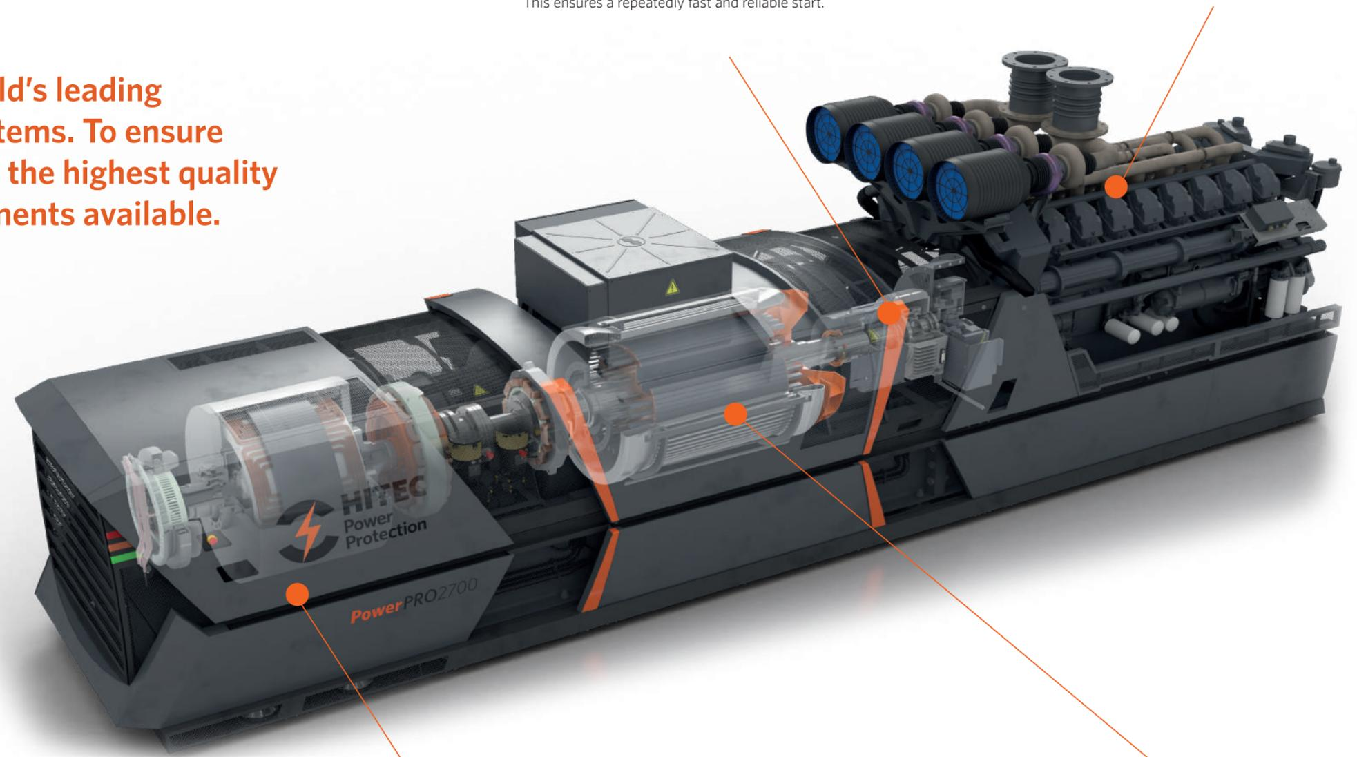
The **FREE-WHEEL CLUTCH** is the mechanical interface between the generator and the engine. The clutch allows the shaft of the generator to rotate while the engine is idle. When the engine starts and the speed of the engine reaches the speed of the generator, the clutch engages automatically, and the engine starts to drive the generator. As a result, the engine starts and ramps up completely without load. This ensures a repeatedly fast and reliable start.
